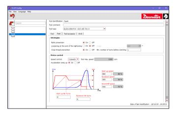
Starting at the start signal, the tool runs with a programmed acceleration up to Rundown speed. The tool keeps running at Rundown speed. Once the number of turns has been reached, the speed changes to Downshift speed.
