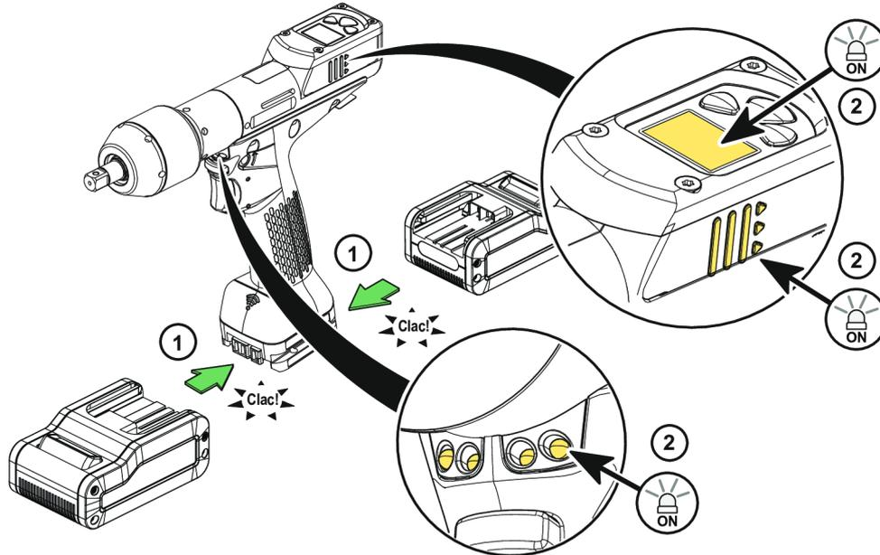
Insert the battery pack in front or behind the tool until a locking sound can be clearly heard.
